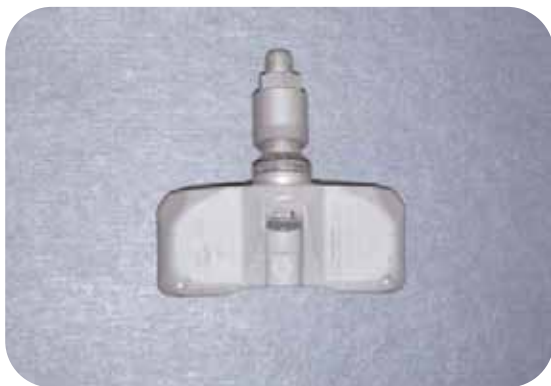
Figure 4C Clamp-in TPMS Valve
