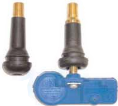
Figure 4A Comparing Standard Snap-In Valve to a TPMS Snap-In Valve with Sensor
